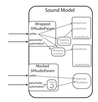
Figure 2: Comparison between the two approaches for wrapping AudioParams
